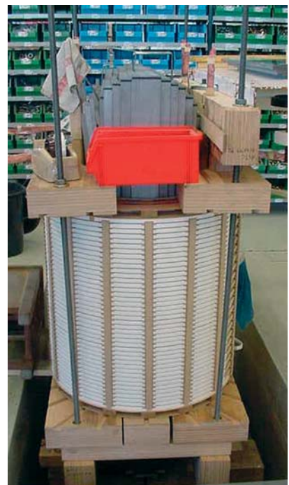
ABB transformer coil insulated with NOMEX® brand paper ready to ship and install.
